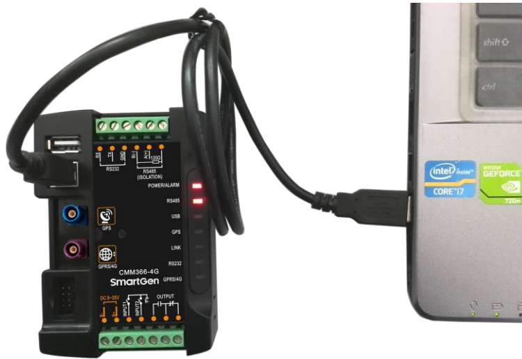
Fig.9 USB and PC Configuration Connection
