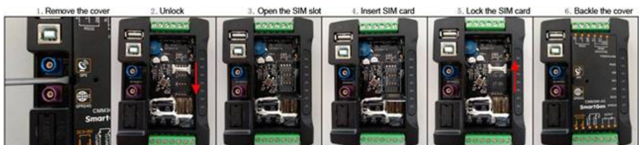
Fig.3 SIM Card Installation
