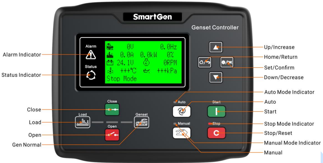
Fig.1 – HGM6110LT Front Panel Indication
