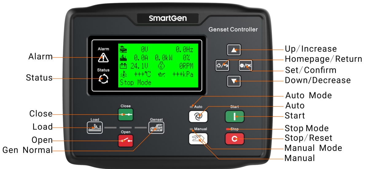
Fig.1 – HGM6110 (HGM6110N/NC/CAN) Front Panel Indication
