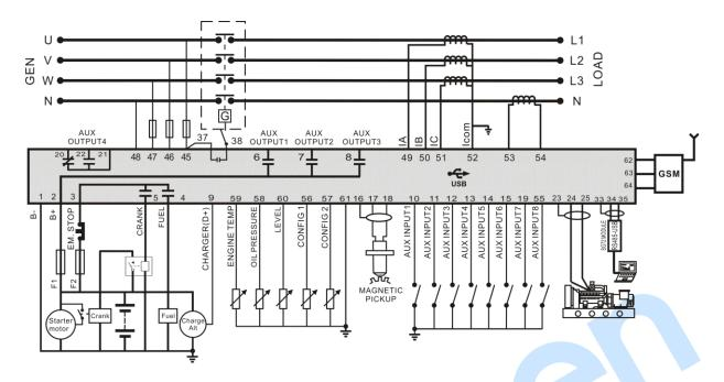
Fig.5 HGM9310MPU(CAN) Typical Application Diagram
