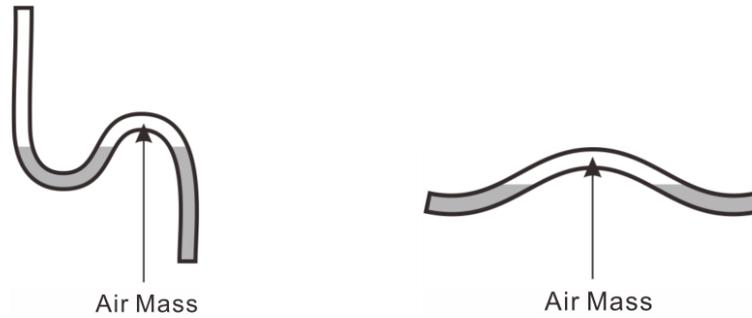
Fig. 4 – Incorrect Pipe Connection Methods
