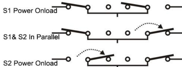
Fig. 3 - Sync Transfer Diagram
