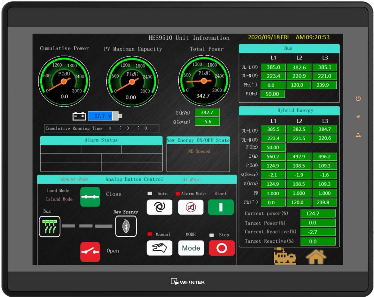
Fig.4 - HES9510 Genset Information of Controller Display
