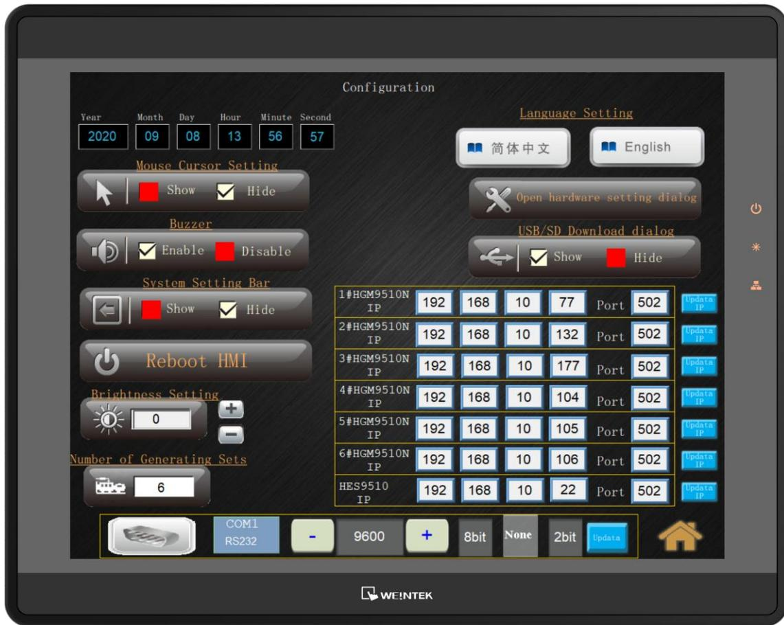
Fig.5 - System Configuration Interface Display
