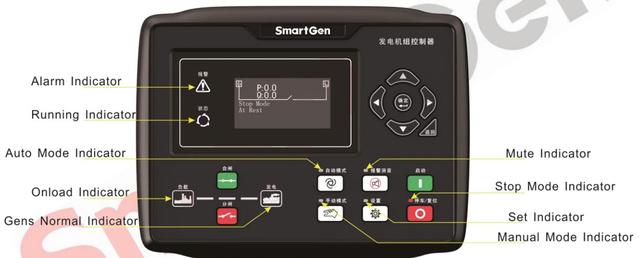
Fig. 1 - Controller Front Panel
