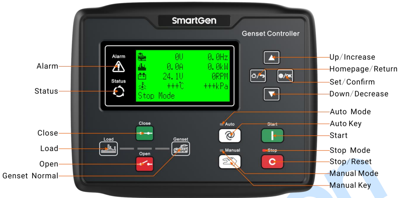
Fig.1 – HGMS61D Front Panel Indication
