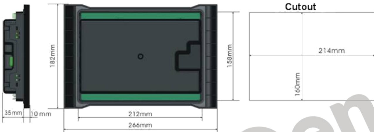
Fig.21 - Installation Dimensions
