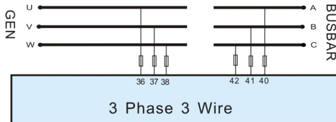
Fig. 5 – 3 Phase 3 Wire Connection
