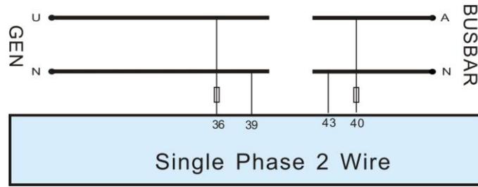
Fig.6 – Single Phase 2 Wire Connection
