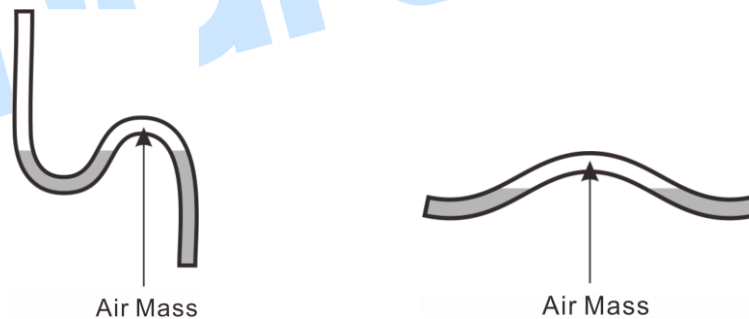
Fig. 3 – Incorrect Pipe Connection Methods
